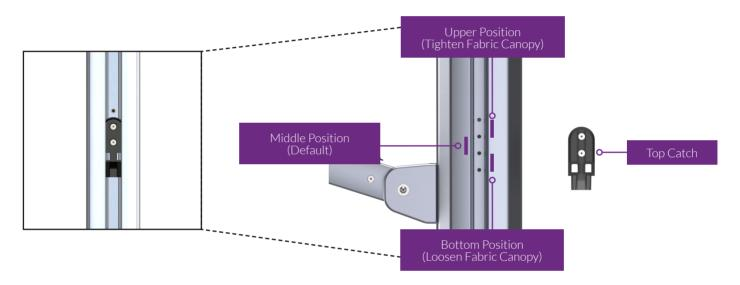
Note: The Top Catch can be moved to adjust the tightness of your canopy. The Middle position is the factory default position, the Upper Position will tighten the canopy and the Bottom position will loosen the Fabric Canopy.
